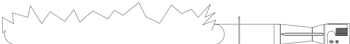
Poor Combustion:wavy,yellow flames-too little air
